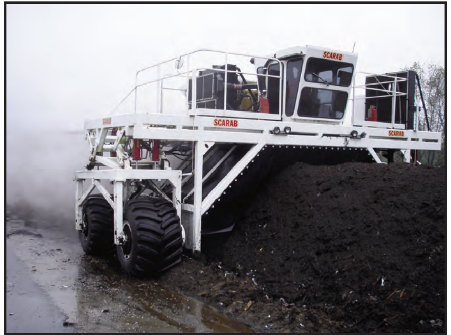
A Scarab machine turns the leaf windrows as it passes over. The steam is a result of the heat contained in the decaying leaf piles.
